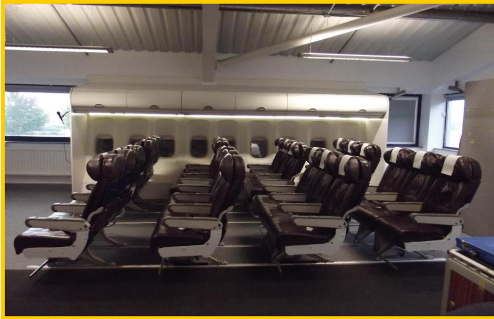
Example of a four row Midi-mock-up cabin and central aisle within a classroom
