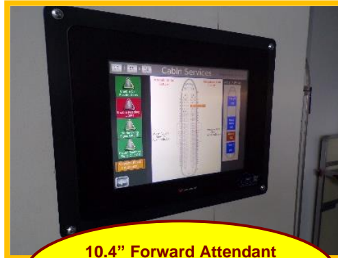
10.4" Forward Attendant Panel/HMI – controls the cabin electronics system
