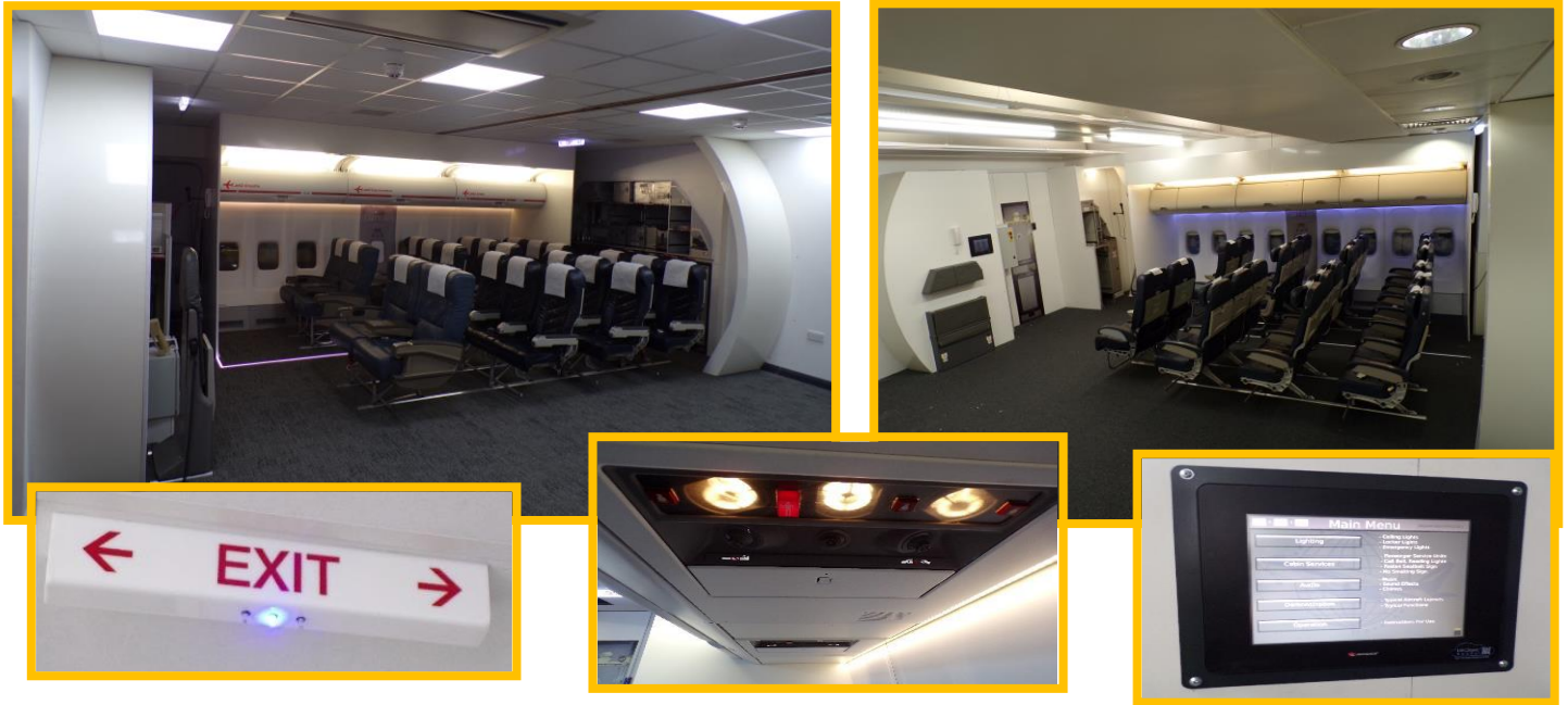
Example of a Cut-away four row mock-up cabin within a classroom – this included a rear full width galley, FAP/HMI system, full electronics, PSUs and Exit/ACP indication + lighting
