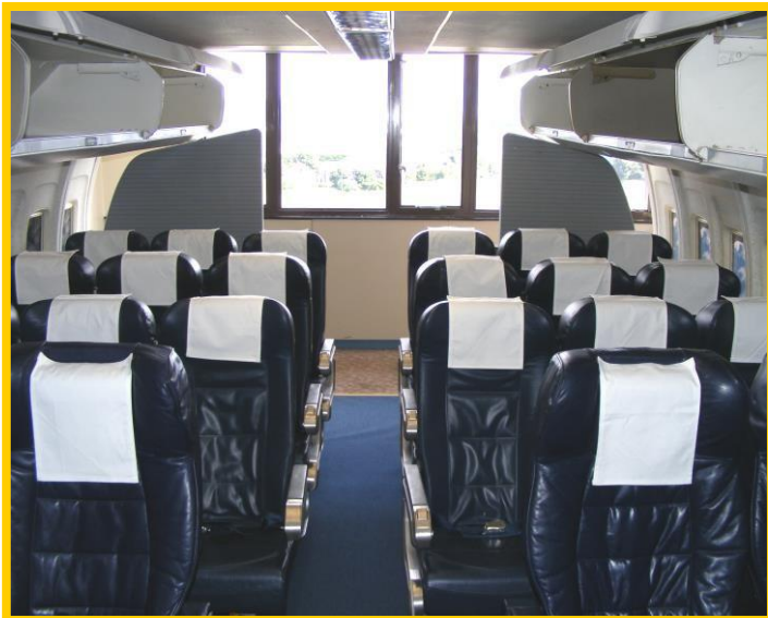
Example of a Cut-away four row mock-up cabin within a classroom – this included a rear full width galley, FAP/HMI system, full electronics, PSUs and Exit/ACP indication + lighting
