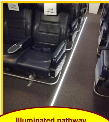
Illuminated pathway marking – controlled by the FAP
